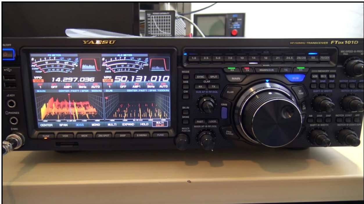
Figure 3: The Yaesu FTDX101D showing dual band reception on the color display
